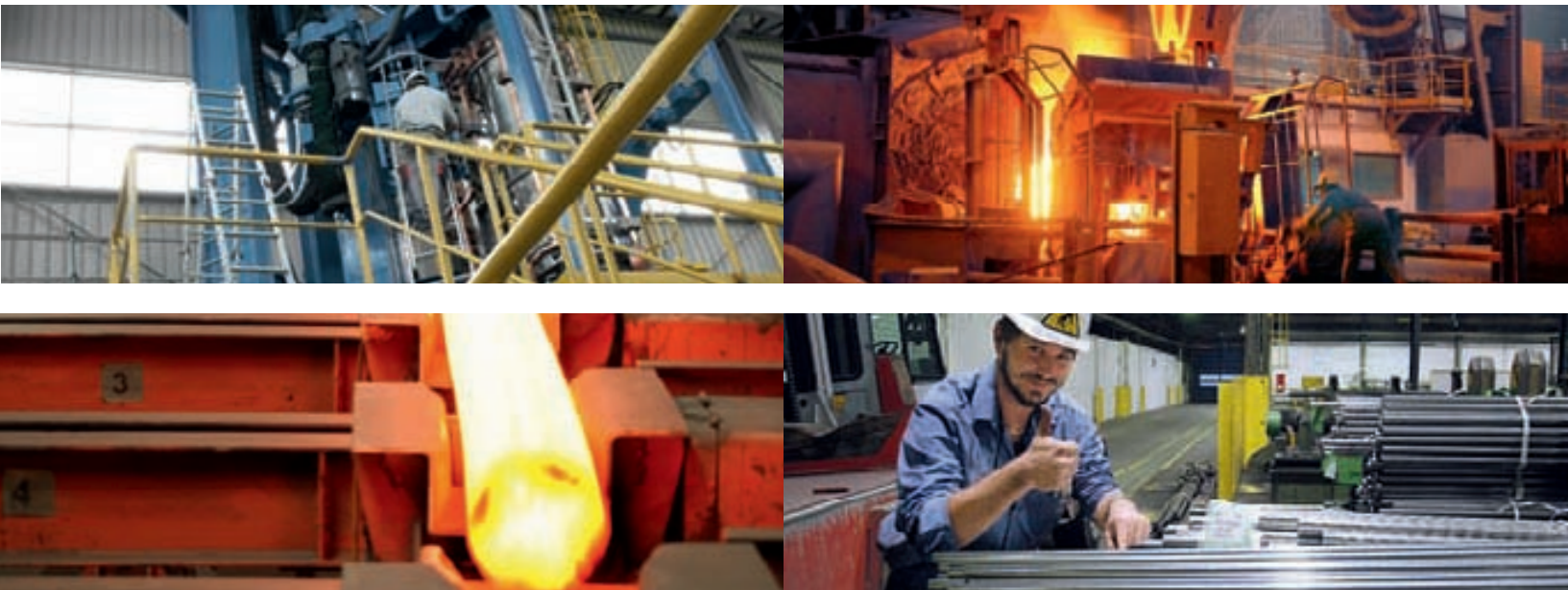
From top left to bottom right: Electro Remelting Slag | Process to blow argon and oxygen in the liquid metal to remove Carbon | Hot rolling mill | Finishing shop storage area
